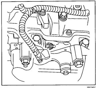
14. Install the cylinder number 2 glow plug harness connector and nut.
