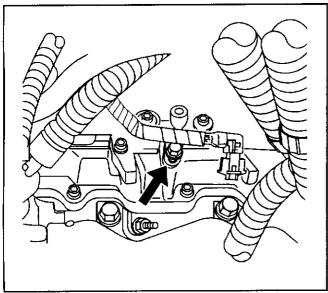
12. Position the new injector harness bracket to align with the bracket bolt hole and secure to the harness with electrical tape.
