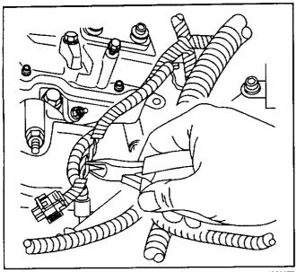
8. Cut cylinder number 2 fuel injector connector off the engine harness approximately 38.1 mm (1.5 in) away from the base of the connector.
