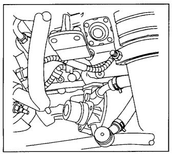
2. Position the fuel filter assembly out of the way.
