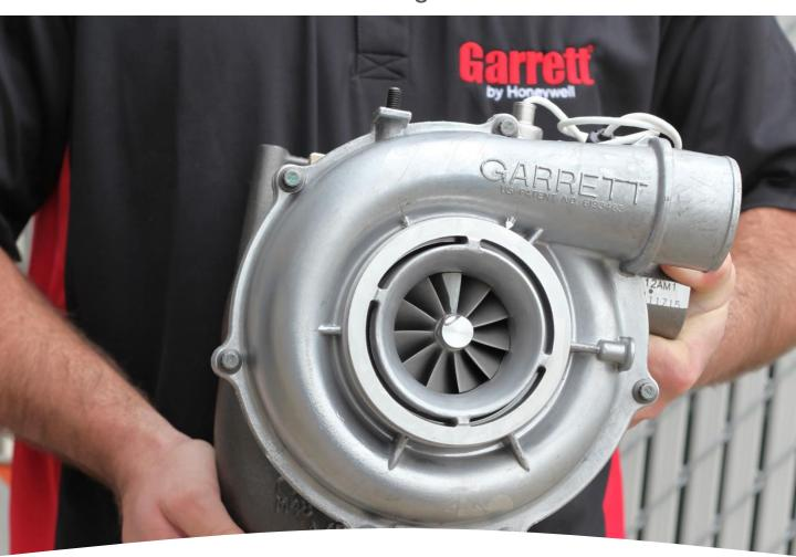
First-fit, Advanced Variable Geometry (AVNT) turbochargers incorporating engineering updates for GM 6.6L Duramax Engines
